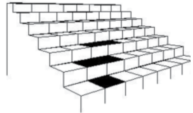
Figure 22. Approximation of a tilted plane by terraces.
