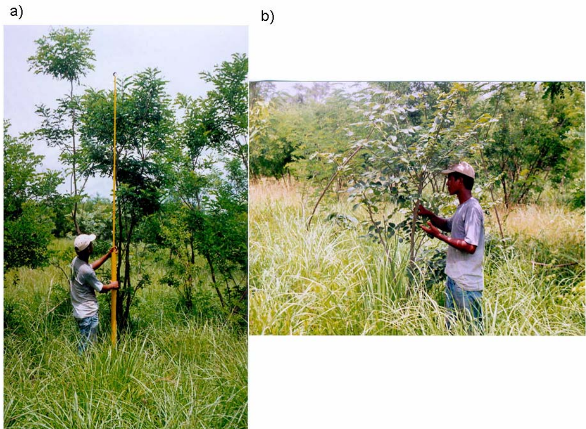
Photo 2. Measurement of tree dimensions a) total height and b) diameter at breast height.
