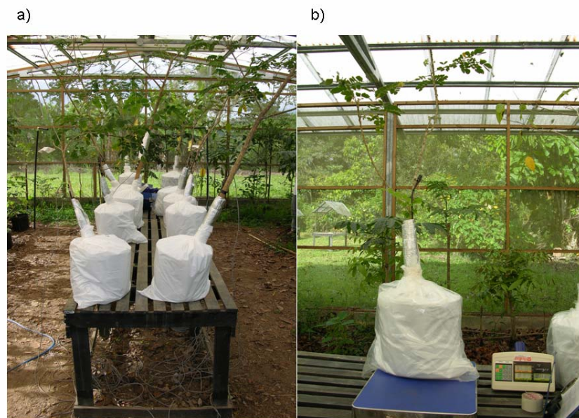
Photo 6. Calibration of sap flow gauges with trees growing in pots in a greenhouse at CATIE: a) general view of trial; b) weighing of pots.
