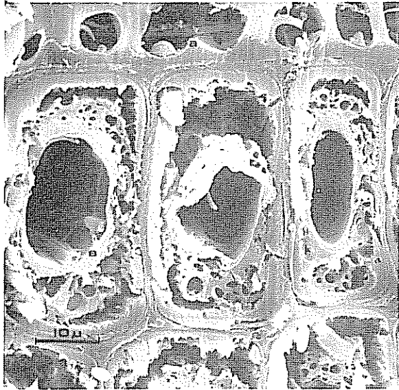
Fig 4 An enlarged cross section of southern yellow pine sapwood invaded by a soft-rot fungus ( Phialophora sp.) showing a hypha transversely penetrating the cell wall (a) and hyphal filaments lining the inner lumen wall (b) SEM Mag 1950 X
