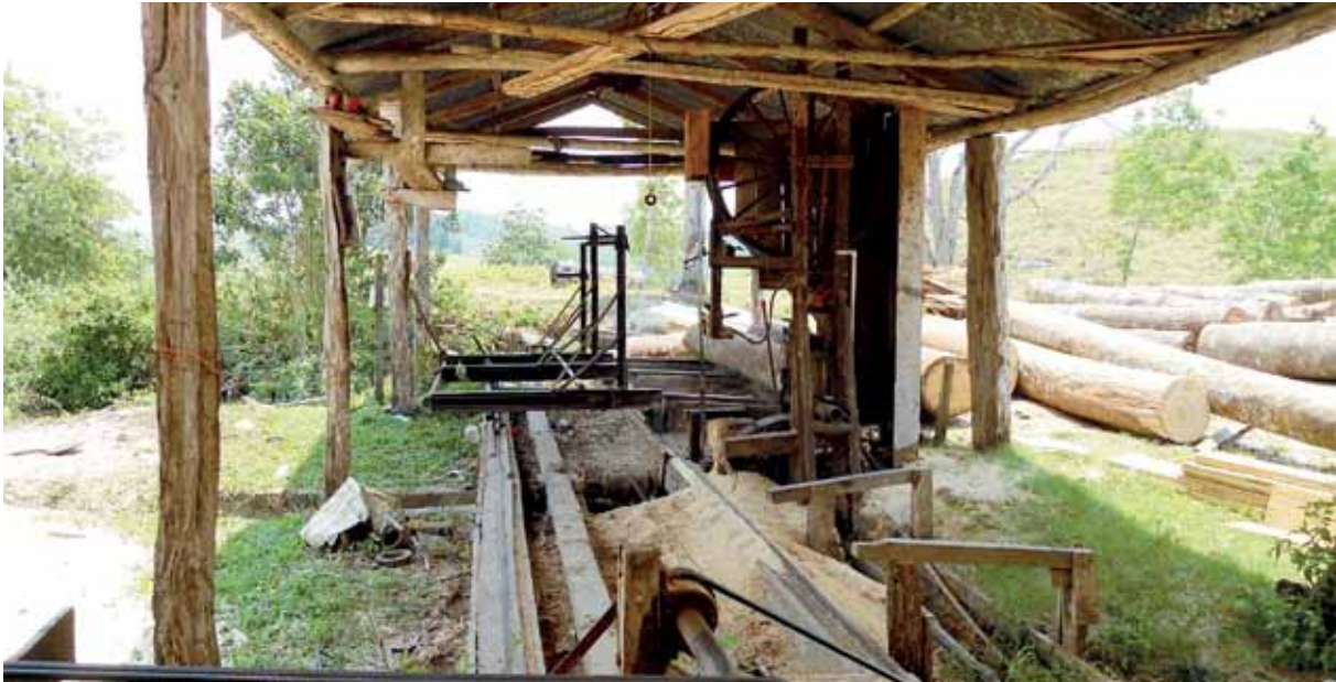
Photo 3. Primary transformation: sawmill machinery form Upper Barton Creek
