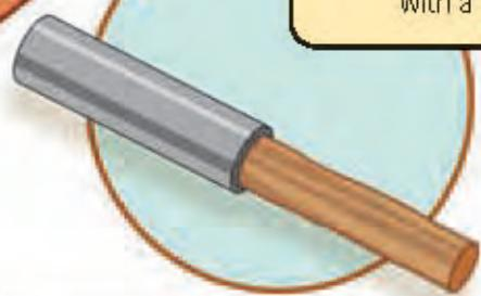
The mallet can be made with a piece of hardwood, coated and protected with a metal tube.
