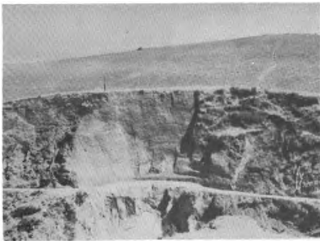
Fig. 12 A construction cut at Ccorimarca Draw showing deeply weathered shales over which mature upland slopes have developed.
