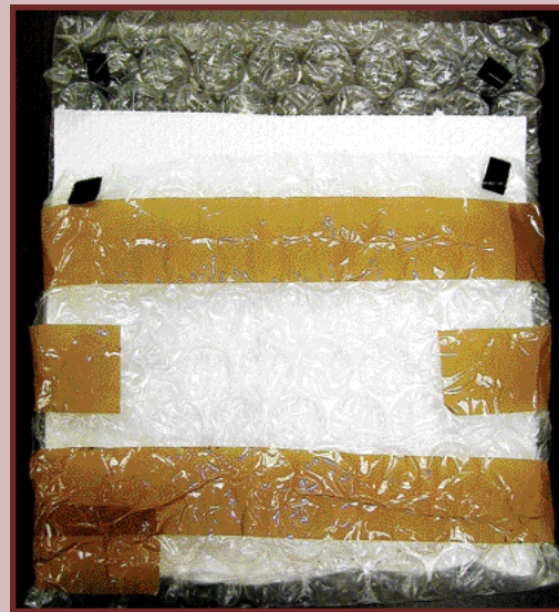
Figure 1: Pod transport bags made from heavy-duty bubble wrap (1.3 cm bubble height) sheet held together with plastic packaging tape. Paper towels were placed in the bags to absorb water transpired by the pod during transport. Bubble wrap sheets were recycled packaging materials shipped with lab supplies
