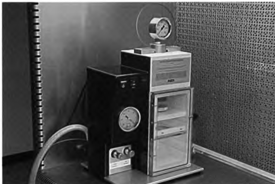
Figure 34. Particle acceleration device utilized at CATIE for biolistics experiments.
