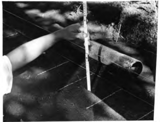
Fig. 3. Second layer of the sampling profile ready for extraction of soil cores. Note marked area which is at a depth of 20 cm from the taut base-line wire.
