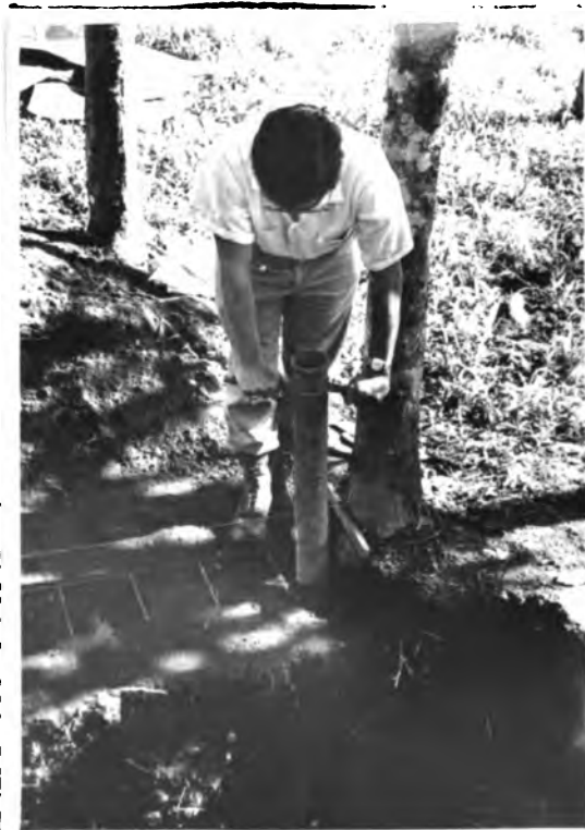
Fig. 4. Method used for the extraction of one-liter core samples from the soil profile.
