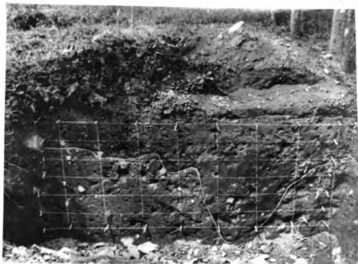
Fig. 5. Soil profile T - 1 The irregular white line marks the limit between humic and non-humic soil layers. Rectangles are 20 x 40 cm and their top limit is 20 cm below the original soil-line.
