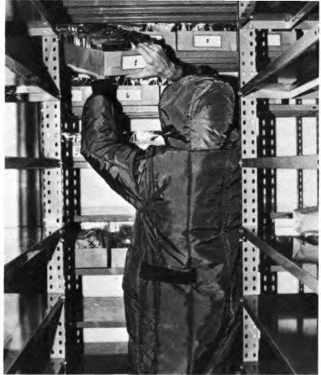
The cold room at CATIE for long term storage of seeds at -20^{\circ}\text{C} .
